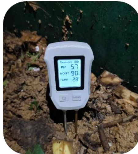
Gambar 2. Pengecekan rutin suhu Sludge hasil IPAL
